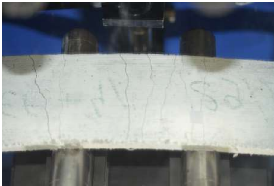
Figure 4. Experimental cracking pattern of composite plate
