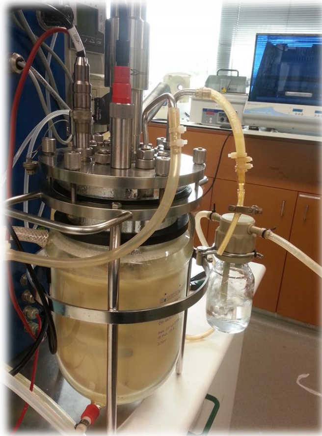
Figure 5 RALF PLUS SOLO bioreactor working with biotransformation medium.
