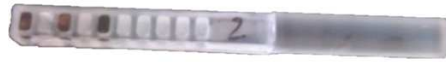
Figure 2.9: Example of a tube with three compartments filled with a certain particle amount. The compartments have a length of 2 mm and are separated by a spacing of 1 mm. In total ten compartments can be used for the representation of various particle distributions. When it is used in the calibration procedure a single compartment is filled.
