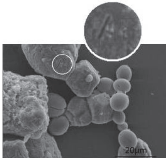
Figure 1: contrast between the large volume of \text{CaCO}_3 crystals and the size of precipitating bacteria as shown by their highlighted imprints (Xu et al. 2015).
