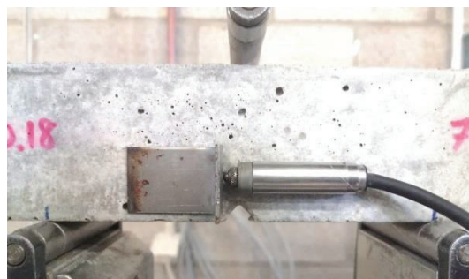
Figure 66: LVDT positioned at the side face of a specimen to measure the crack size at the height of the embedded capsule.
