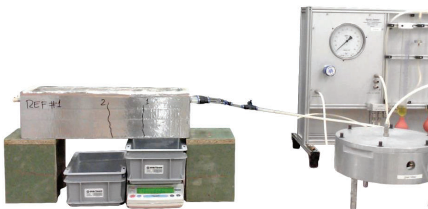
Figure 80: test setup for determination of water flow through cracked planes.
