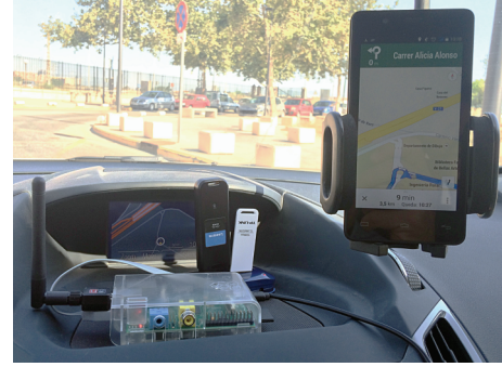
FIGURE 1: A GRCBox hardware module formed by a RaspberryPi and 3 WiFi interfaces: one in access point mode, one in station mode, and one in ad hoc mode.
