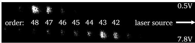
Fig. 3.26: Recorded laser diffraction pattern of the hybrid blazed grating at two different voltages. The location of the beam incident on the reflective grating, relative to the reflected beam, is indicated in the figure, as well as the order number, m , of each of the diffraction orders.
