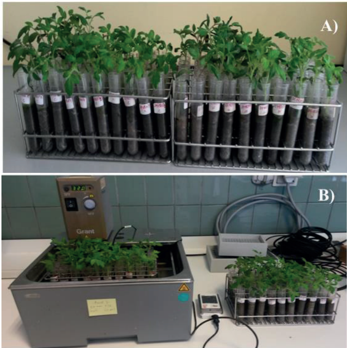
Figure 5.1. A) Plastic tubes with tomato seedlings; B) the experimental set up for the heat stability test in a warm water bath with simultaneously recording of the soil temperatures using a data logger (TESTO).
