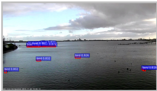
Fig. 11. CNN Py-faster object detection with COCO dataset shows the feasibility of CNN based bird/water classification .
