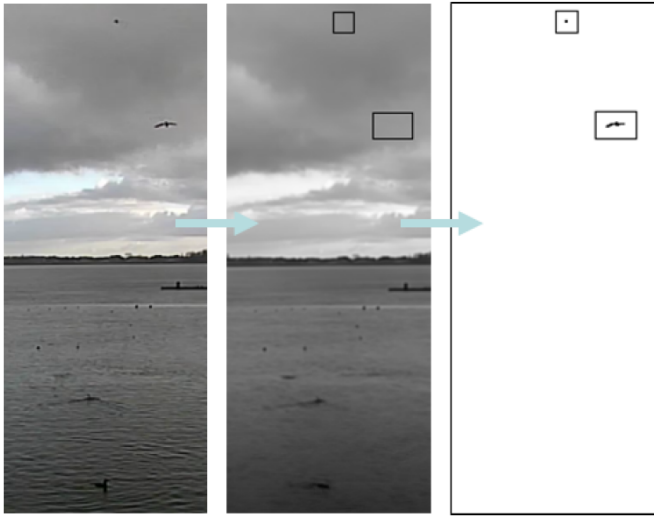
Fig. 4. Results of the proposed dynamic background subtraction. Flying birds are more easily found than birds resting on the water surface. Different background model updating and thresholding approaches are investigated.
