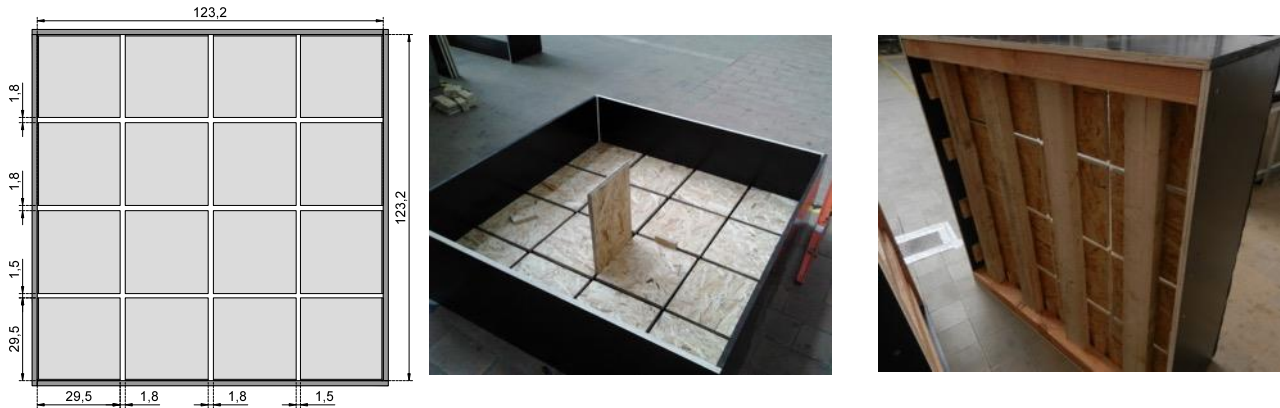
Fig. 1: Test setups: left: dimensions of the setups in cm; middle: 16 panels screwed onto structure; right: wooden structure surrounded by framework at the back of the test setup
