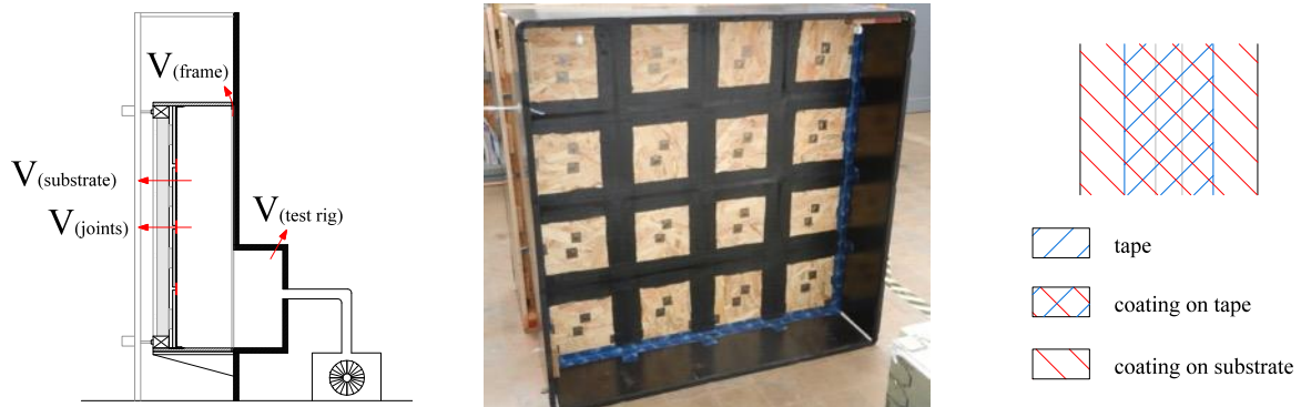
Fig. 2: Calculation of air leakage sealed joints; left: different air leakages through test setup; middle: covered joints; right: covered part of substrate
