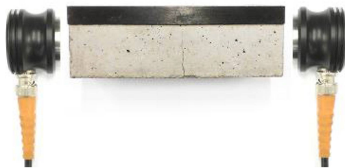
Figure 1. Specimen configuration with a single crack at mid-span and a reinforcing FRP strip; US shear sensors are attached at opposite sides.
