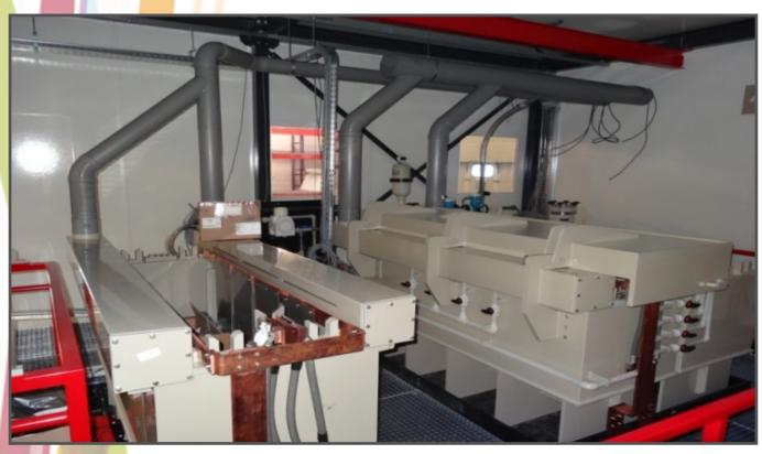
Due to the promising features of this new electrodeposition solvent, a flexible semi-industrial pilot plant has been designed in OCAS NV. In this way, several set-ups, IL compositions, additives, etc. can be tested and evaluated on a large scale, and compared with lab scale experiments.
