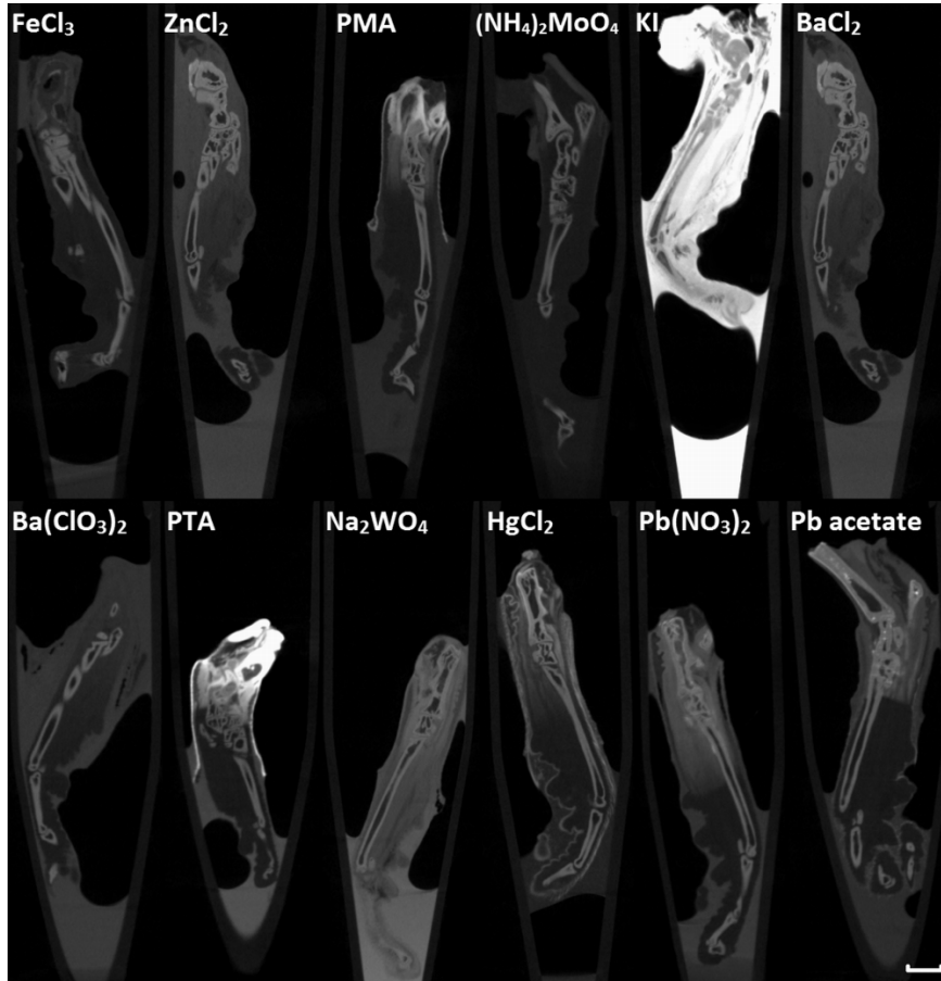
Figure 5.8: Sagittal CT slices of the mice paws illustrating the penetration depth after 24 hours staining. The contrast agents are indicated on the figure. Scale bar = 2.5 mm [1].
