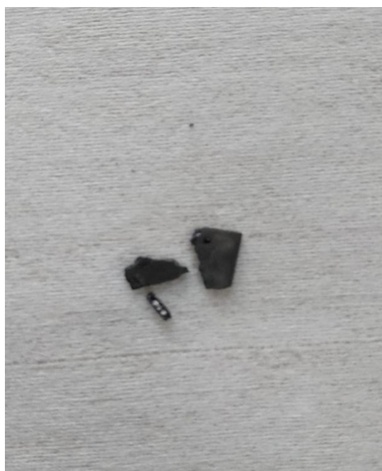
Figure 6. Broken Ti-base alloy coupon after cracking pretreated at 1273 K.
