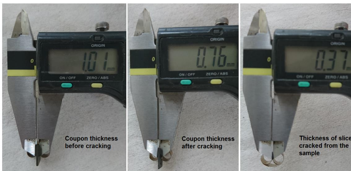
Figure 5. Thickness values of the Ti-base alloy before cracking (left), after cracking (middle) and of a broken slice (right), pretreated at 1173 K.
