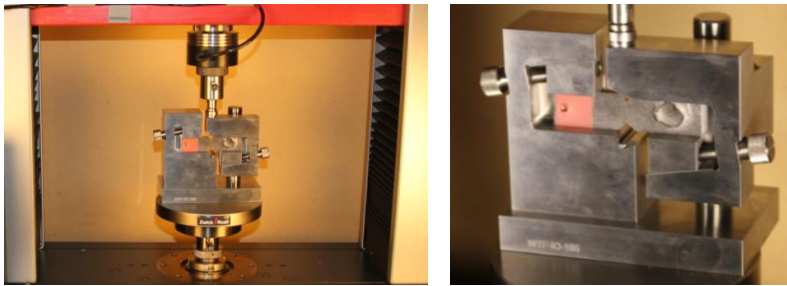
FIGURE 3.25: TEST SETUP OF THE IOSIPESCU SHEAR TEST
