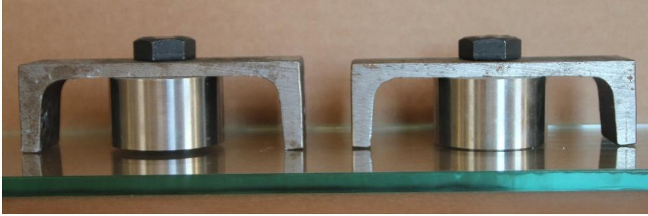
FIGURE 4.4: EXAMPLE OF THE BRACKET WITH A CONNECTOR OF \varnothing 50 MM FOR THE MS-POLYMER SO (LEFT) AND THE 2C-EPOXY 3M (RIGHT).
