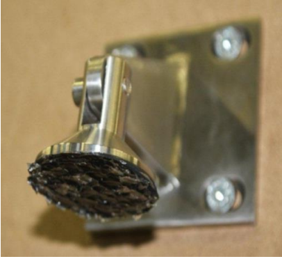
FIGURE 2.14: DETAIL OF CONNECTION AFTER FAILURE WITH A THIN LAYER OF BROKEN GLASS STILL ADHERED TO THE ADHESIVE (BELIS ET AL. 2012).
