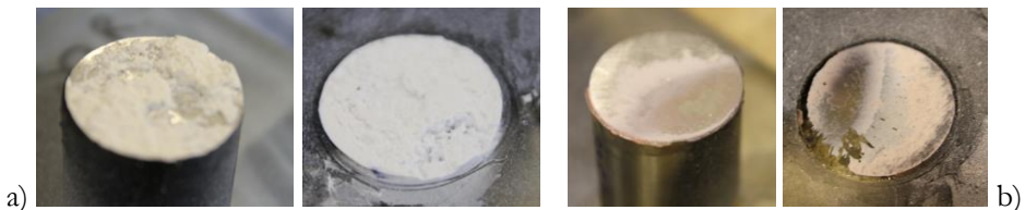
FIGURE 8.11: FRACTURE SURFACES OF COHESIVE FAILURE WITH A) SOUDASEAL 270 HS AND B) 3M™ SCOTCH-WELD™ 9323 B/A.
