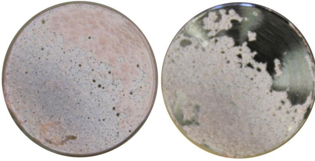
FIGURE G.6: FOAMY FRACTURE PATTERN FOR SERIES E-3M.
