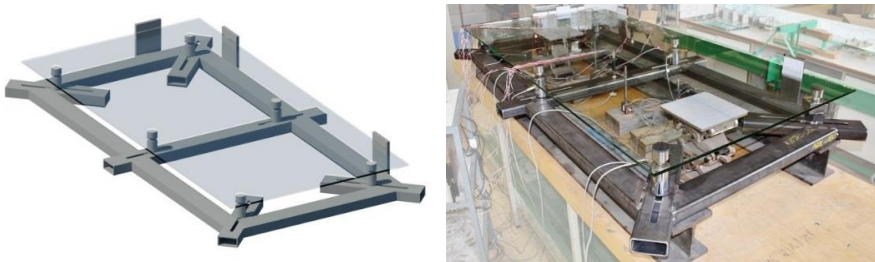
FIGURE 6.2: GRAPHIC REPRESENTATION OF THE EXPERIMENTAL CONFIGURATION AND THE ACTUAL EXPERIMENTAL CONFIGURATION FOR SIX POINT-FIXINGS WITH A DIAMETER OF 50 MM.
