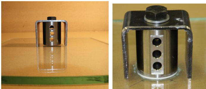
FIGURE 4.33: EXAMPLE OF THE BRACKET FOR THE MS-POLYMER SO WITHOUT ADHESIVE (LEFT) AND WITH ADHESIVE (RIGHT).
