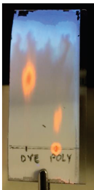
Figure S22. Reversed phase TLC of free Rho dye (left) and PTX-polyDMA 30 -Rho (right) (eluent: 1:1 H 2 O:acetonitrile v/v, 1 % TFA).
