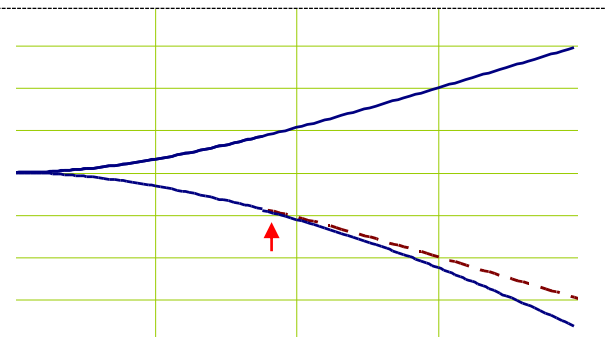
Figure 2. Maximum elongation of a beam with breathing crack near the center.
