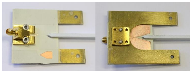
Fig. 1. Photographs of the assembled transition: microstrip side (left) and slotline side (right)
