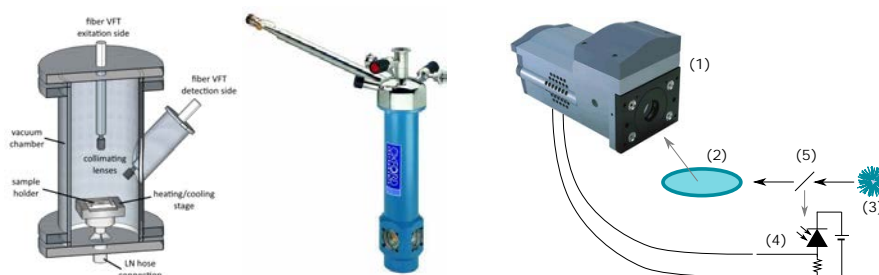
Figure 7.5 – Left: T -TL setup, used to measure thermal quenching [323]. Middle: Cryostat, used for low temperature experiments. Right: ICCD and schematic overview of the experimental determination of decay profiles. The meaning of the numbers is elucidated in the text.
