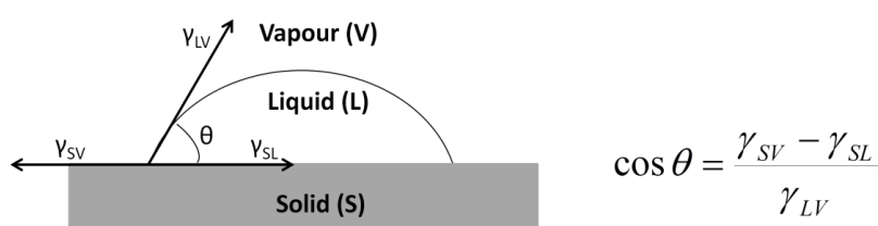
Figure 6.3: Definition of the static contact angle ( \theta ), according to Young's equation.
