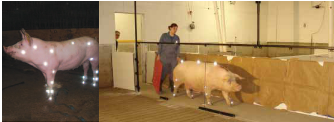
Figure 1.2. Positioning of reflective markers at various anatomical landmarks in a pig (top) prior to kinematic gait analysis (bottom). Source: Newcastle University/Prairie Swine Centre.
