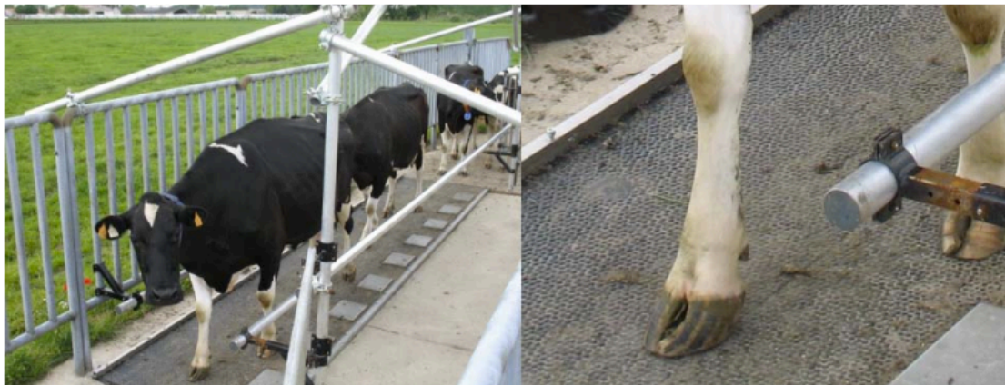
Figure 1.3. Pressure sensitive runway developed by Van Nuffel et al. (2009) to study gait in dairy cattle.
