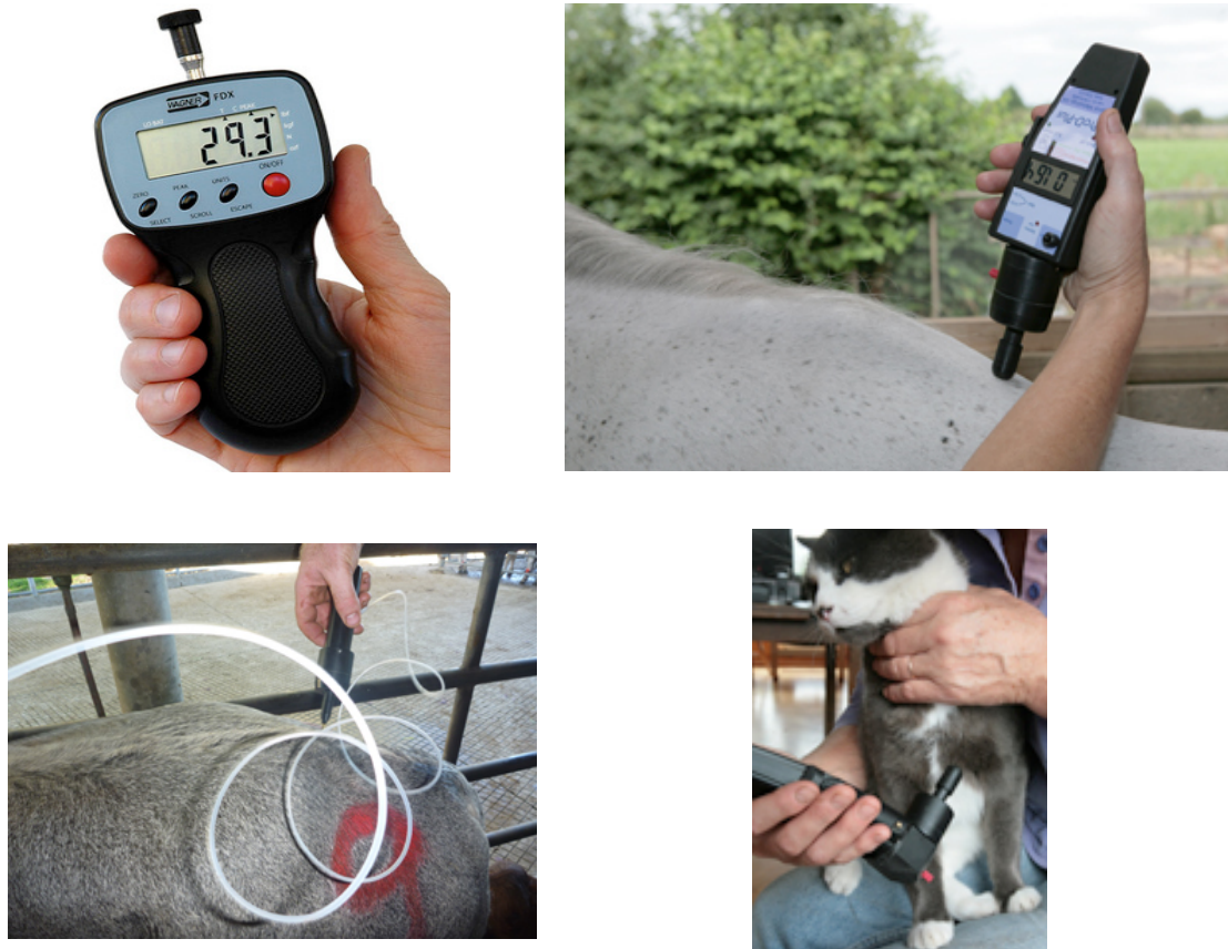
Figure 1.13. Different models of hand-held pressure algometers, for use in small and large animals. The algometer is a force transducer provided with one or more tips of variable materials, shapes and diameters and which is manually pushed against a given anatomical landmark – preferably at a constant rate – until a codified behavioural response is obtained from the animal. The average of several readings at the time of the reaction, either expressed as units of force or pressure, is the mechanical nociception threshold of the landmark tested. Image sources: Top left Wagner Instruments. Top right, bottom left and right: TopCat Metrology.
