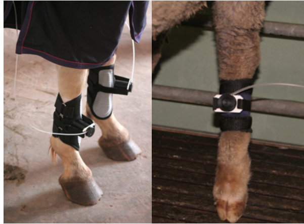
Fig. 1.14. Limb-strapped pneumatic devices connected to a digital algometer with tubing for remote measuring of mechanical nociceptive thresholds. The pressure within the plastic tube pushes the pin within the pneumatic device against the skin of the animals at a constant rate, until a behavioural response is obtained. At that point, pressure can be manually removed and the pin immediately retracts. Source: TopCat Metrology.
