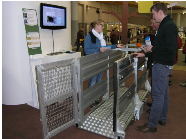
Figure 1.5. The SowSIS measuring device described in Pluym et al. (2013). The the bottom plate contains four force plates that continuously record force stance variables, once the sow is standing inside the modified crate. Visual stance variables are also recorded with a mounted photcamera.
