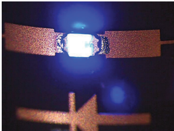
Figure 4. Optical micrograph of a powered LED after photonic soldering on a PET flex foil using a 200 ms modulated pulse with 16 \text{ J/cm}^2 energy.
