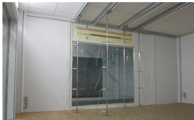
Figure 3. Hot box with prototype vent above the window and automatically moving measuring grid in the room.
