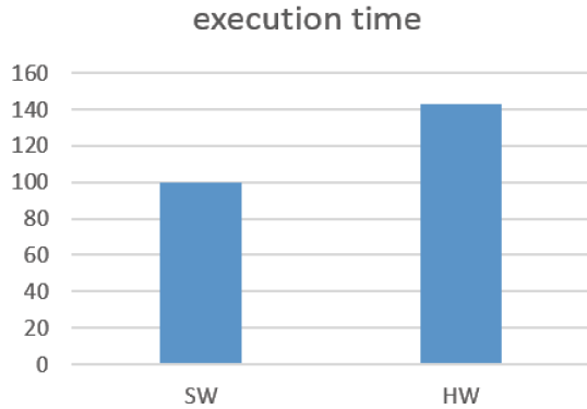
Fig. 13. Execution time of the software and hardware implementations of the Raytracing algorithm.
