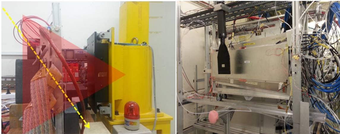
Figure 3. Prototype RPCs installed at a distance of 36 cm from the 5.55-GBq ^{137}\text{Cs} source at Korea University (left), and at about 5 m from the 13.9-TBq ^{137}\text{Cs} source at the GIF++ (right).
