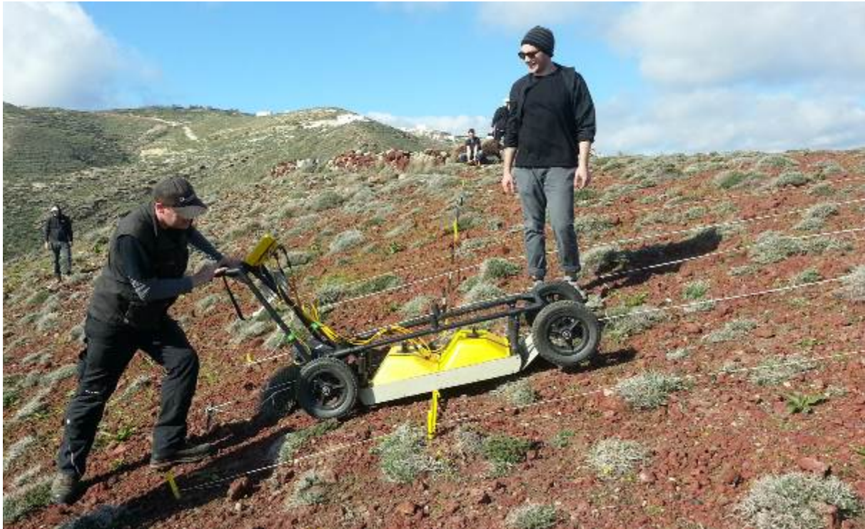
Figure 1 Ground penetrating radar measurements with a 250 MHz antenna system and 25 cm profile spacing on top of Kokkino Vouno (Red Mountain) near the archaeological site of Akrotiri. Photo: Klaus Löcker.
