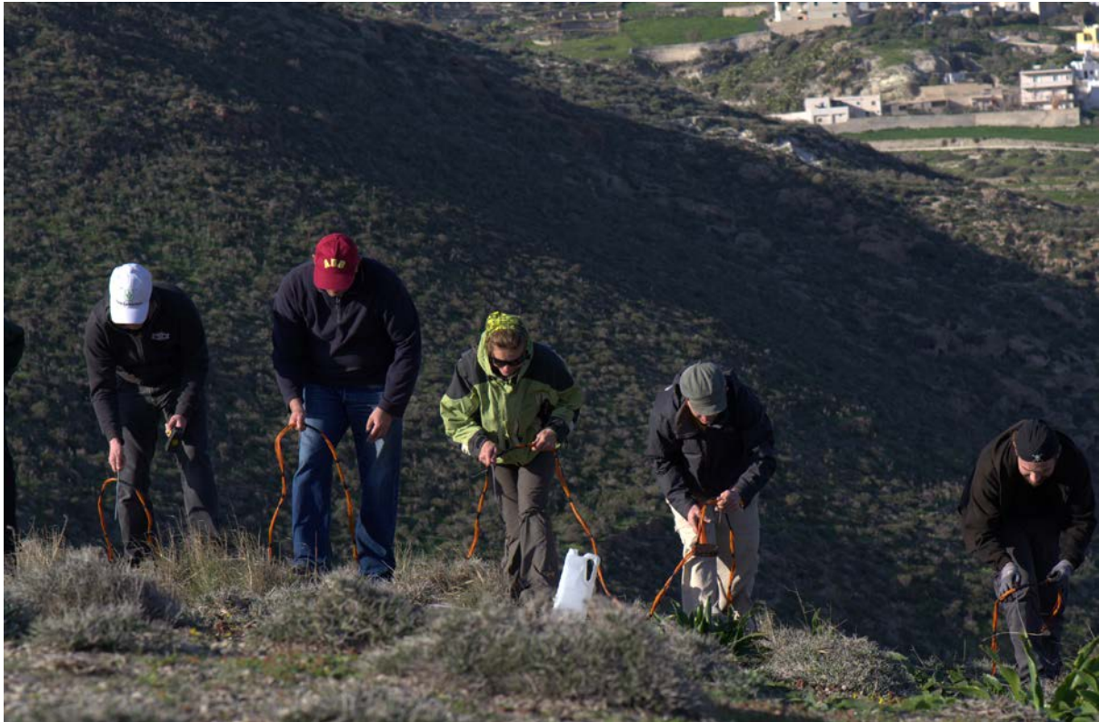
Figure 3 Moving the electrodes on the Red Mountain for Electrical Resistance Tomography measurements. Photo: Geert Verhoeven.
