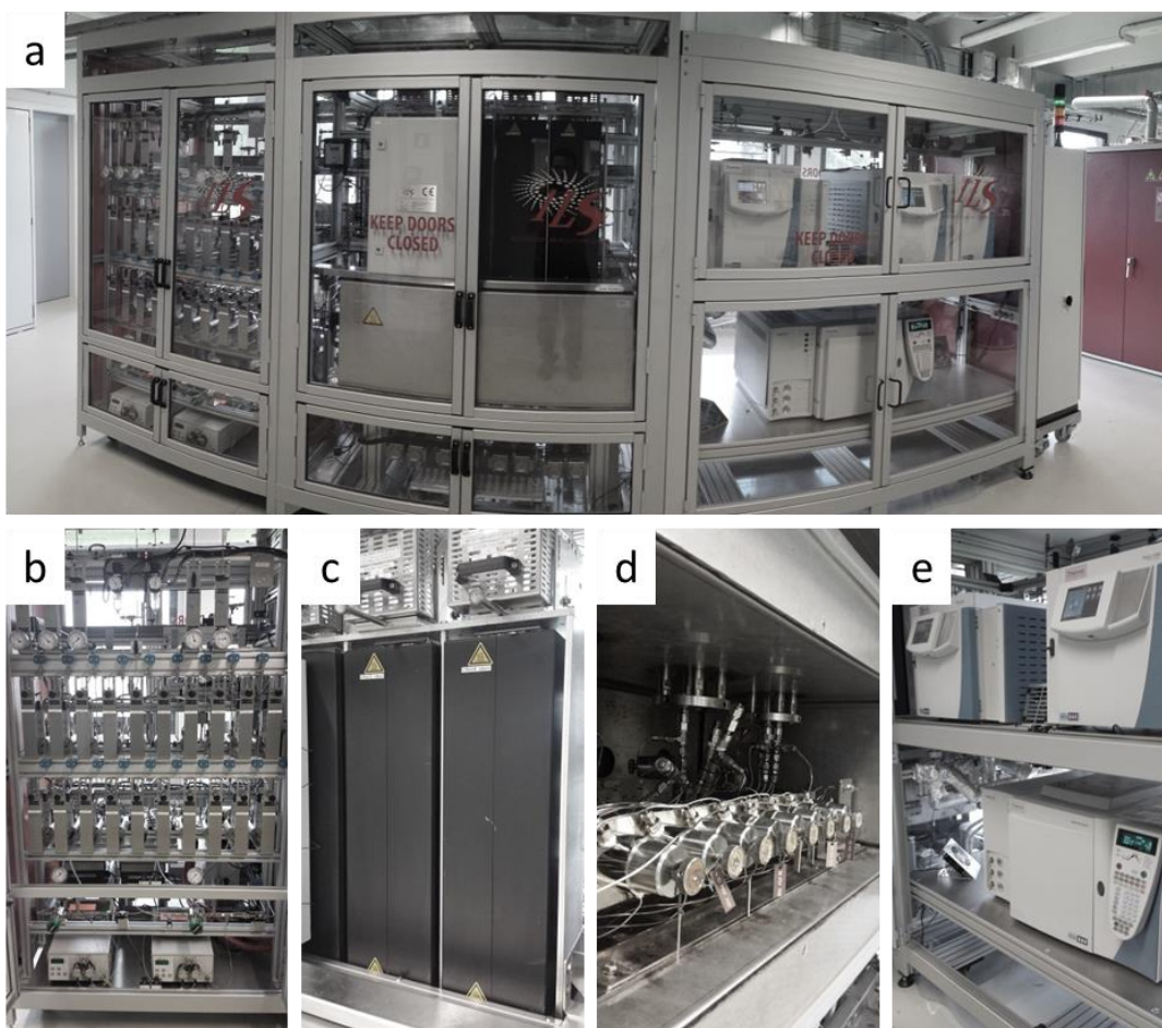
Figure 2-3: HTK-S set-up pictures: a) front view, b) gas (top) and liquid (bottom) feed section, c) reactor heating blocks, d) heated gas and liquid sampling section and e) analysis section
