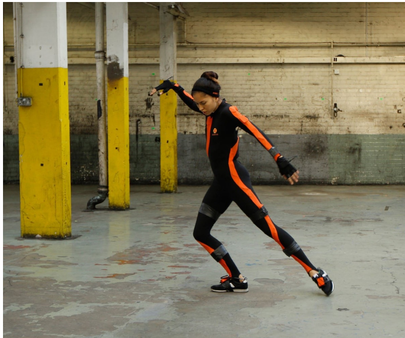
Figure 51. The Xsens suit used in the creation process of Wide Open (2016). Xsens MVN (or MOVEN) is a full-body, camera-less motion capture solution that detects body movements via inertial sensors attached to the suit. It is a flexible system that can be used indoors or outdoors (on-set).
