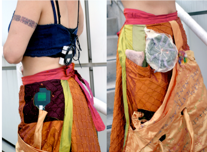
Figure 46. Breath sensing technology integrated in costumes for the performance exhale . Left. LED array embedded within fabric to display continuous breath data. Right: exhale breathband measures breath, while RFID tag enables breath exchange.
