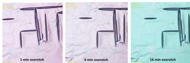
Figure 3.5 (a) Micron-sized defects can be seen in the device layer after the substrate removal has finished. (b) Overetching these defects does nothing to remove them.
