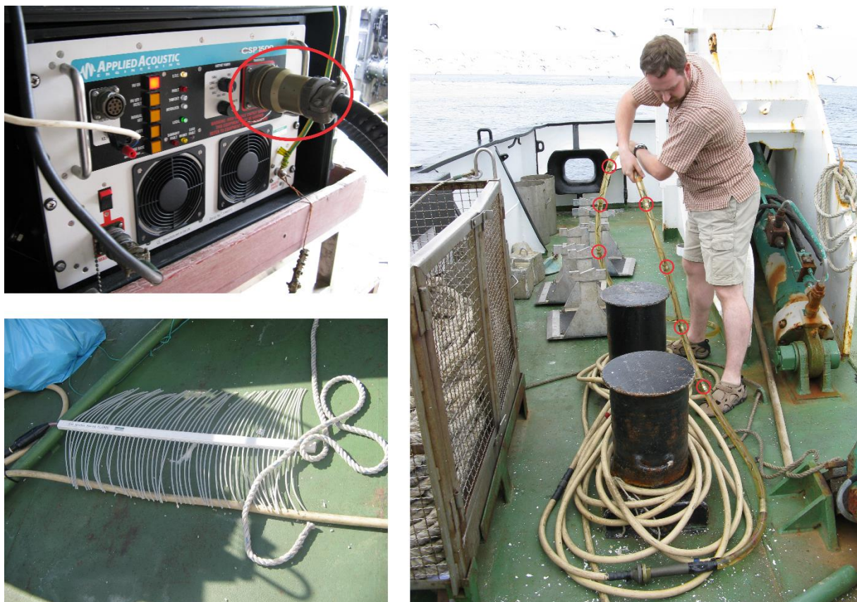
Figure 3.1: Components of the sparker system. Upper left: power supply with the cable towards the sparker indicated. Lower left: Sparker containing 100 electrodes. Right: streamer with 10 electrodes (red), each 0.5 m apart.
