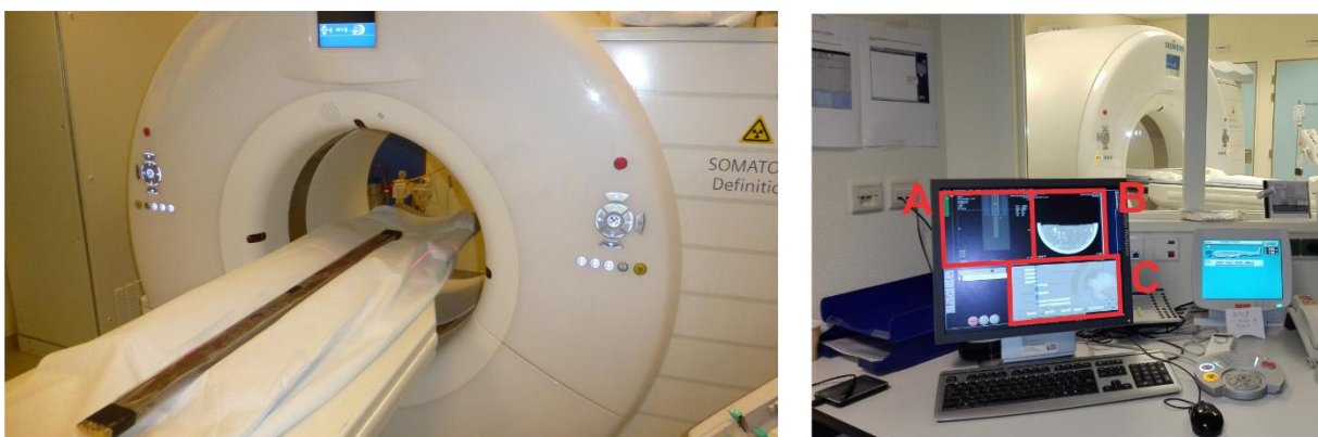
Figure 3.10: Left: Sediment core on the scanning table. The source and detector are positioned within the cylinder and rotate around the sample. Right: view on the acquisition software, with radiograph (A), individual slice (B) and input parameters (C). Pictures courtesy of Maarten Van Daele.
