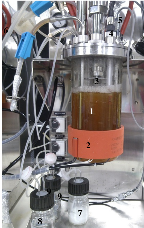
Fig. 2-1 experimental set up of submerged fermentation of A.oryzae ; (1): fermentation culture, (2): external jacket, (3): impeller shaft, (4): PH sensor, (5): DO sensor, (6): air filter, (7): anti-foam, (8) alkaline, (9): acid.
