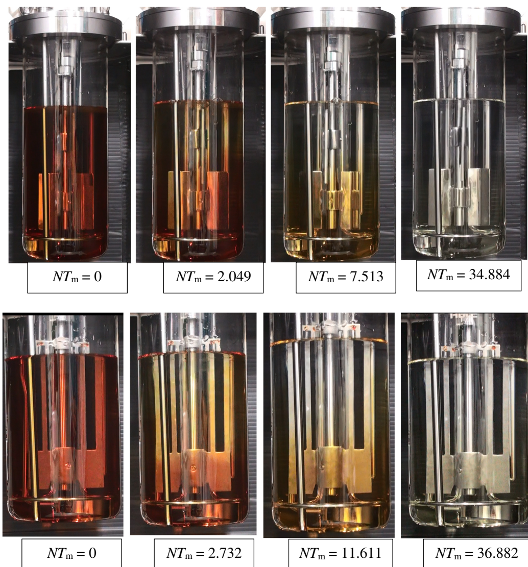
Fig. 4- 6 Results of mixing time measurement using FZ and MB impellers by discoloration method at the same power consumption ( P_v = 150 \text{ W/m}^3 ).
