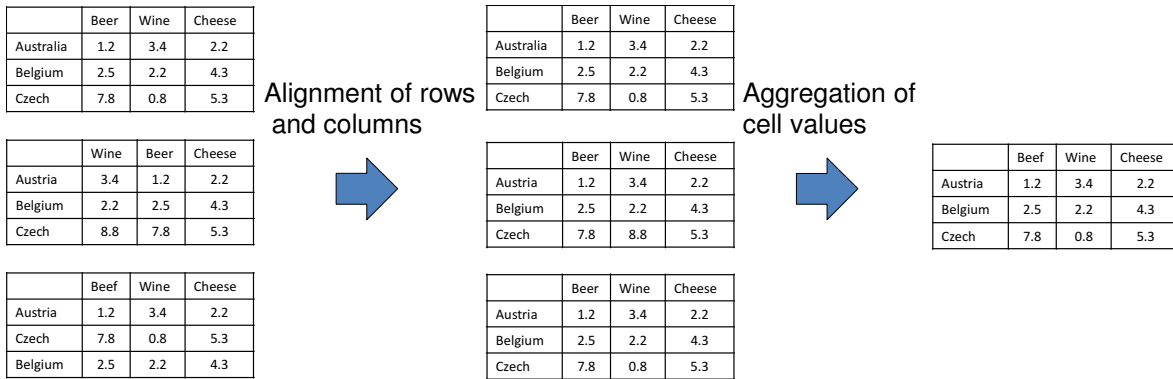
Fig. 7. Example of aggregating tables created by three workers. After the rows and columns are aligned, the corresponding values from the three tables are integrated to obtain a single table.
