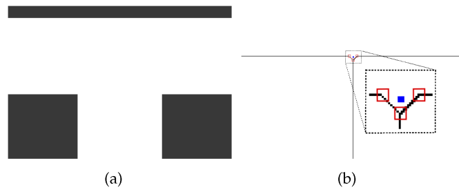
Figure 2. Node extraction from a skeleton map: (a) a map with obstacles and free space; (b) a corresponding skeleton map. Nearby nodes are clustered to form a single node.
