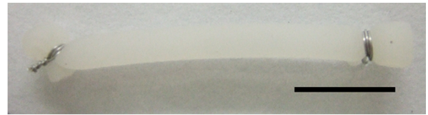
FIG. 5. An example of the sample tubing used to measure the rate of evaporation of water. The tube was filled with double-distilled water. The sample shown is LMP-TPE tubing. The scale bar is 10 mm.
