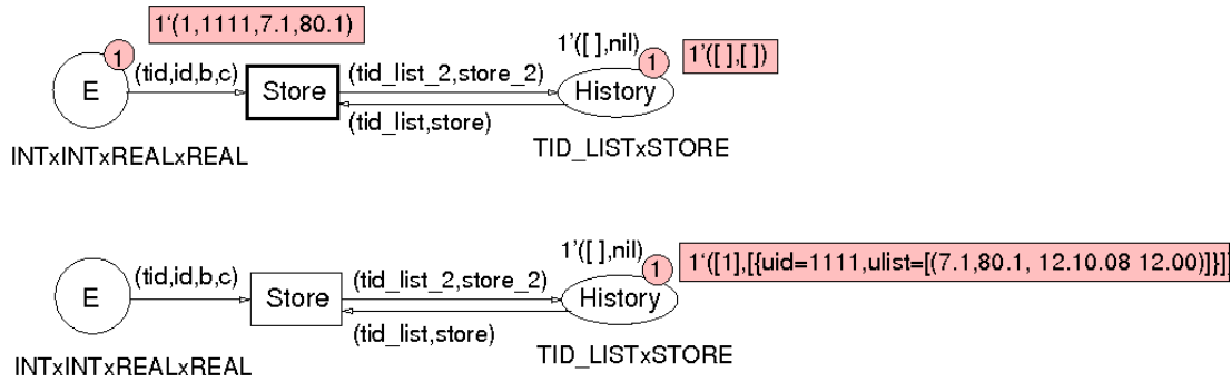
Figure 2.26 – Picture detail of 2.25: storing metered data in history.
