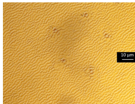
Fig. 2. Differential interference contrast (DIC) optical microscope image of the deteriorated surface of a sample with Si 2 H 6 /TMIn molar ratio equal to 15.27 \times 10^{-5} .
