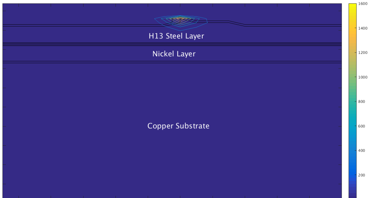
Figure 4 Temperature distribution in transverse cross-section of the sample during SLM of third layer of H13 steel (super-imposed on the material distribution)
