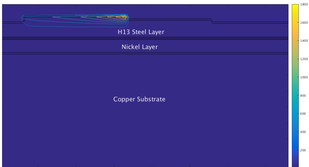
Figure 3 Temperature distribution in longitudinal cross-section of the sample during SLM of third layer of H13 steel (super-imposed on the material distribution)
