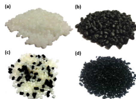
Fig. 1. (a) PA 6,6, (b) MWCNT filled masterbatch, (c) hand mixed masterbatch/ PA6,6, and (d) nanocomposite product of twin screw extruder.
