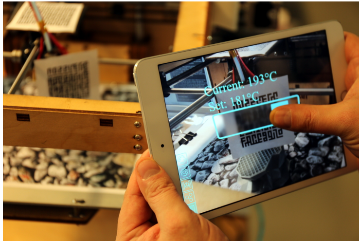
Fig. 4. A minimal augmented interface showing the target and current temperatures of the heated print nozzle. Additionally a slider is included for easy manual operation.
