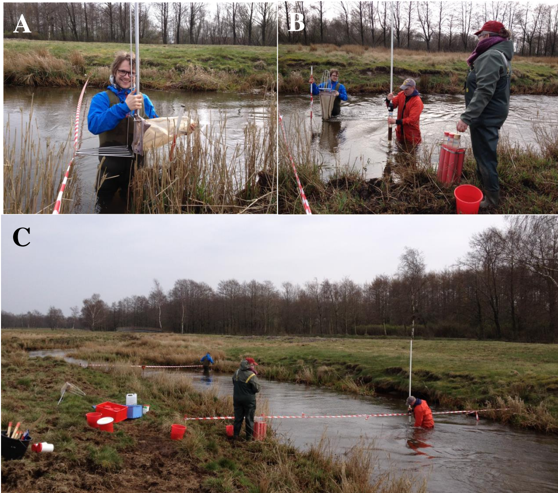
Figure 6. First, (A) macroinvertebrate sampling was conducted using a 500-cm 2 surber sampler along each of the three transects at 25%, 50%, 75% and 100% from the stream bank. Secondly, (B) streambed sediment was sampled along each of the three transects by taking kayak cores in triplicate (Kronvang et al., 2003). (C) Demonstration of the sampling along the transects at station 3 in April 2014. For the detailed sampling strategy, see Figure 5.
