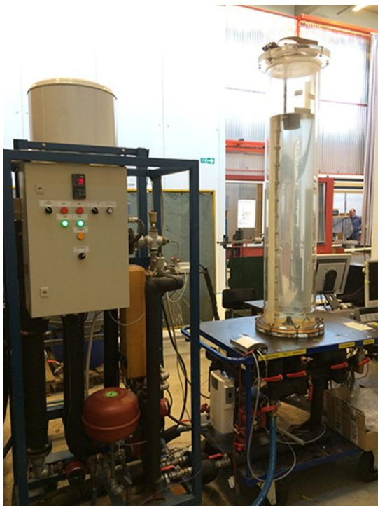
111 112 Figure 1. Photo and schematic sketch of polymer test tank with an inlet stratifier connected to a heat storage test 113 facility. The tank has 15 temperature sensors.
