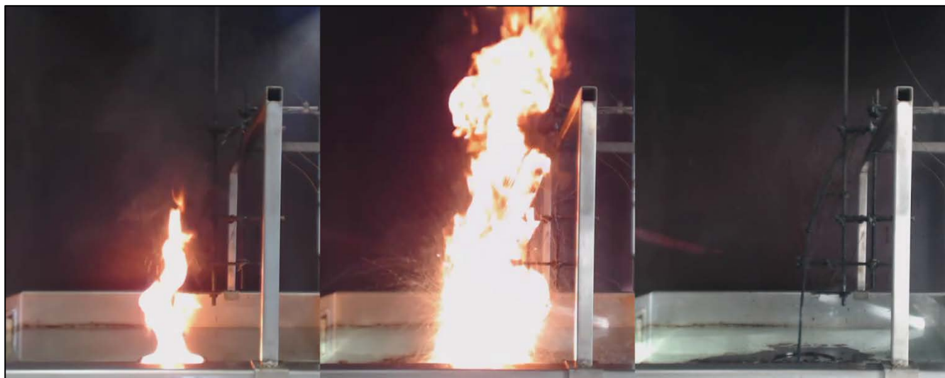
Figure 4.28. Regular burning of REBCO (left) followed by a boilover (middle) and the resulting spreading of the residue, after flame extinction (right). The frames are 77 cm wide and 91 cm high.
