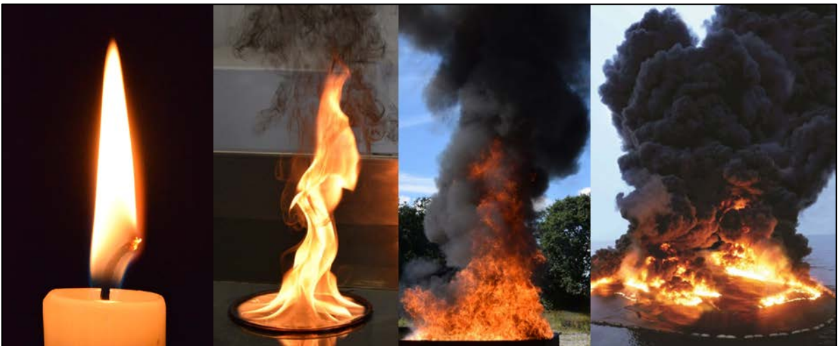
Figure 2.2. Examples of the flame type and smoke production for a laminar candle flame ( D = 7 mm), a laminar-turbulent small scale fire ( D = 0.16 m), a turbulent intermediate scale fire ( D = 1.5 m) and a turbulent operational scale fire ( D > 10 m). Operational scale photo (right) by Elastec (Allen, 2016).
