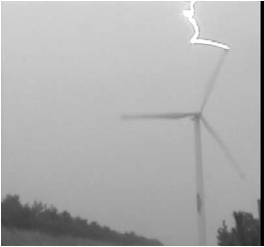
Figure 1. Typical upward lightning on WT. The plasma channel is swept due to the angular velocity of the tip receptor.
