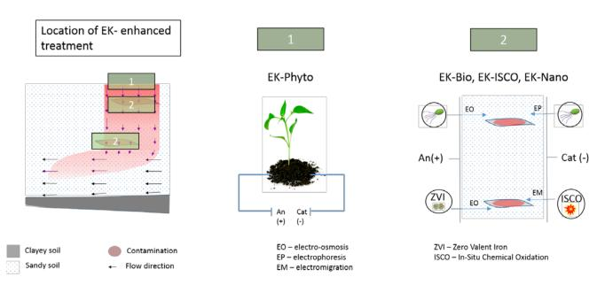
Figure 2 – Schematic representation of electrokinetically enhanced remediation. The left most scheme shows where, within the subsurface or underground, which EK-enhancement would be better suited. Scheme 1 (middle frame) represents the combination of EK with phytoremediation. Scheme 2 (right frame) summarizes how EK would enhance/transport/aid bioremediation, ISCO and nZVI applications.
