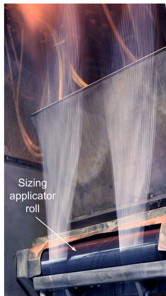
Figure 2.5: Fibres drawn from two bushings passing the sizing applicator roll [20].
