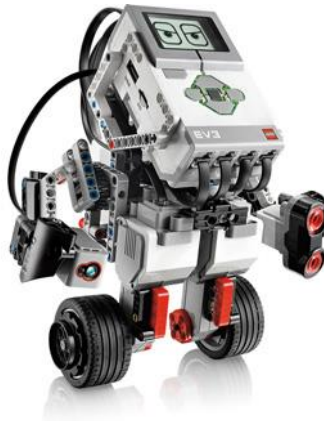
Figure 1: GyroBoy. The robot is 23 cm high and weighs 822 gram.
