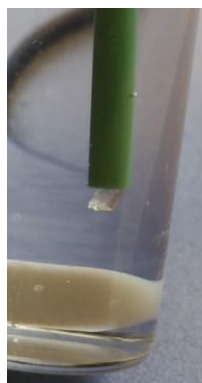
Figure 5. L-arginine crystal blocking the air injection point a few minutes after crash cooling.
