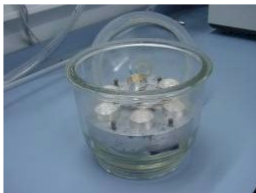
Figure 5.2: Isopiestic measurement performed in glass container
