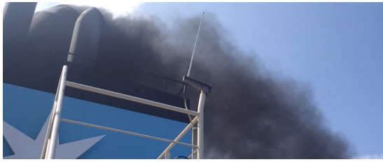
(a) Y_{LA}+PI . Thick black smoke is emitted for 45 seconds.
