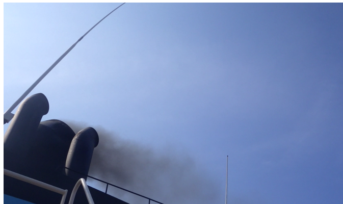
Figure C.14: Exhaust smoke level with adaptive feedforward controller during engine speed step. Gray smoke is emitted for 20 seconds.
