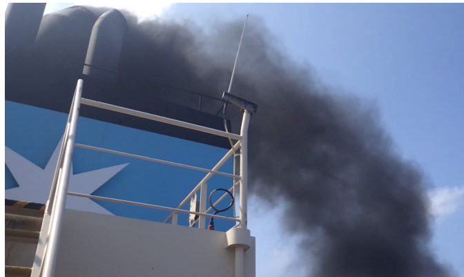
Figure D.3: Exhaust smoke on a vessel with DLF and EGR during engine speed step. Thick black smoke is emitted for 45 seconds. In this test, the Y_{LA} limiter was used in combination with PI EGR control.
