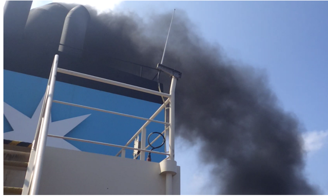
Figure C.13: Exhaust smoke level with PI controller during engine speed step. Thick black smoke is emitted for 45 seconds.
