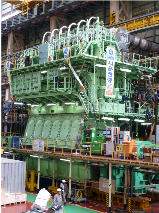
Figure 1.1: MAN Diesel & Turbo 6S80ME engine built by HHI. The engine is being tested before installation on the vessel Maersk Cardiff. The size of the engine can be inferred by comparing to the personnel at the base.
