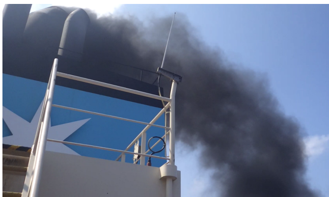
Figure 1.6: Exhaust smoke on the vessel Maersk Cardiff during a large engine load transient. The reference EGR control system was used. Thick black smoke was emitted for 45 seconds.
