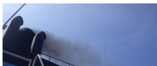
(b) Y_{LA}+AFF . The smoke level is reduced compared to the PI controller but still visible.
