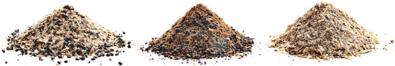
Figure 27: Fuel mixes included in LT-CFB fuel screening. Left) Mix 1 – Palm Kernel Shells & Rice husks, 50/50 w/w, Center) Mix 2 - Palm Kernel Shells & Animal meat and bone meal C1, 50/50 w/w, Right) Rice husks & Animal meat and bone meal C1, 50/50 w/w. All weights on As Received basis.
