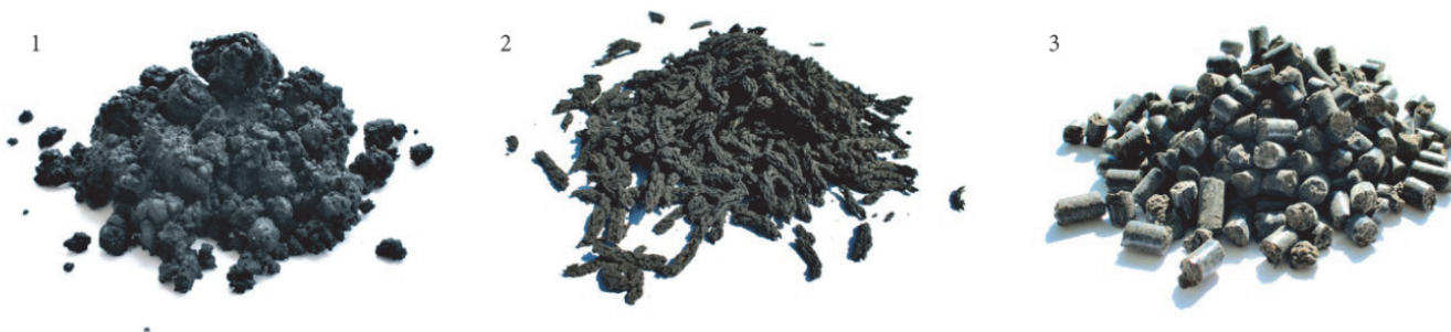
Figure 30: Samples of sewage sludge from three Danish wastewater treatments plants. 1) Mechanically de-watered sludge from Stegholt WWTP, Aabenraa, Denmark (2013). 2) Dry sludge granules from Randers Centralrenseanlæg, Randers, Denmark (2012). 3) Dry sludge pellets from Bjergholm WWTP, Roskilde, Denmark (2015).
