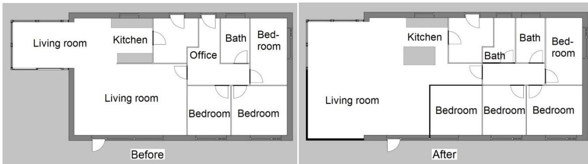
Fig. 8. Layout of House B before and after the suggested changes. The changes were: an extension expanding the living room; removal of the kitchen wall; an extra bedroom; an extra bathroom.
